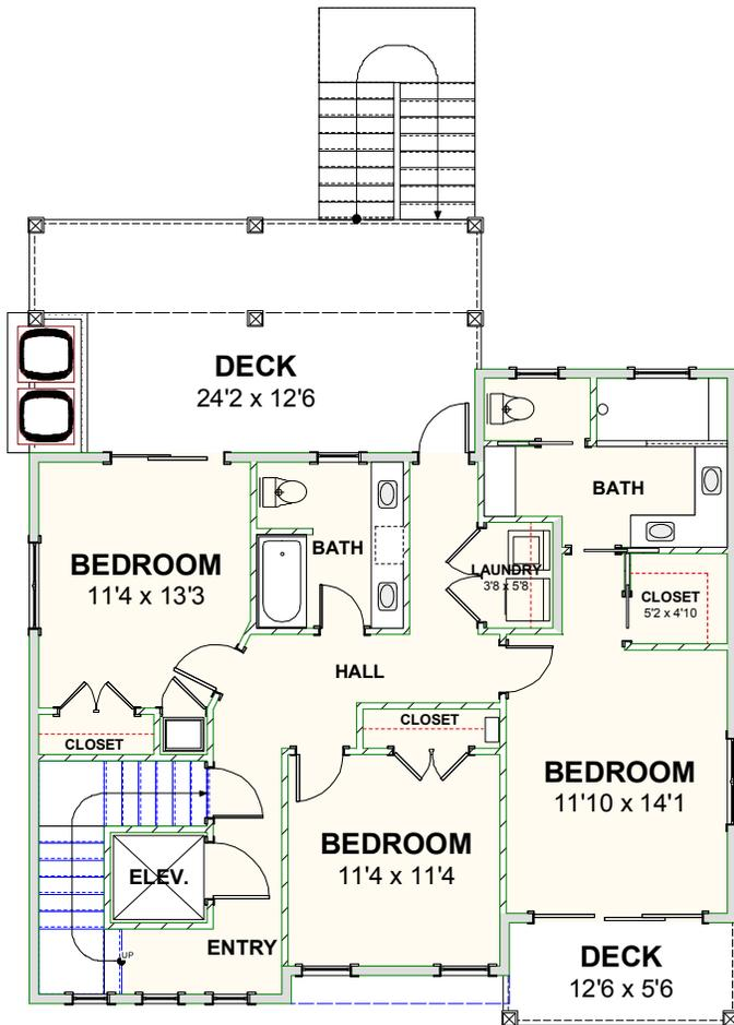
1ST FLOOR - FLOOR PLAN
